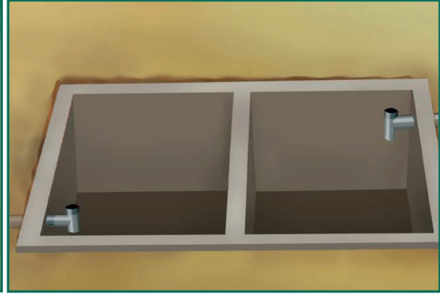
Figure 57 Tanks/chambers lined with T-pipes connected
