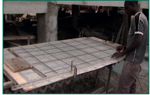
Figure 60 Formwork for pre-cast parts
