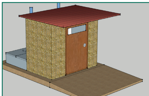
Figure 2 Front view of a KVIP toilet
