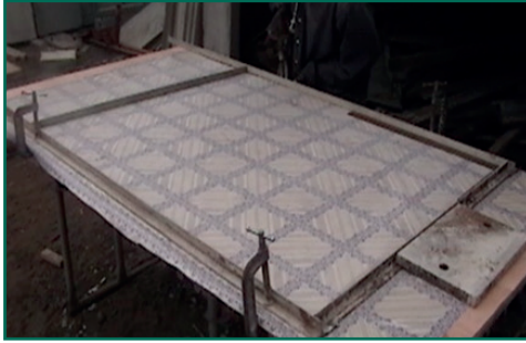
Figure 60 Formwork for pre-cast parts
