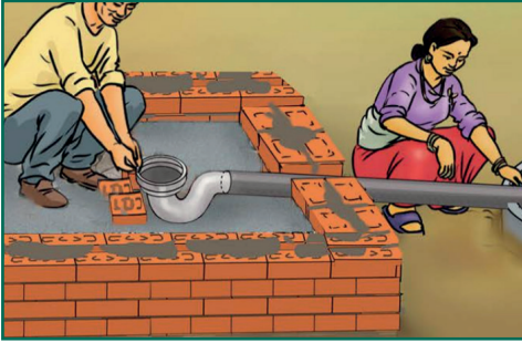
Figure 52 Placing the pipe
